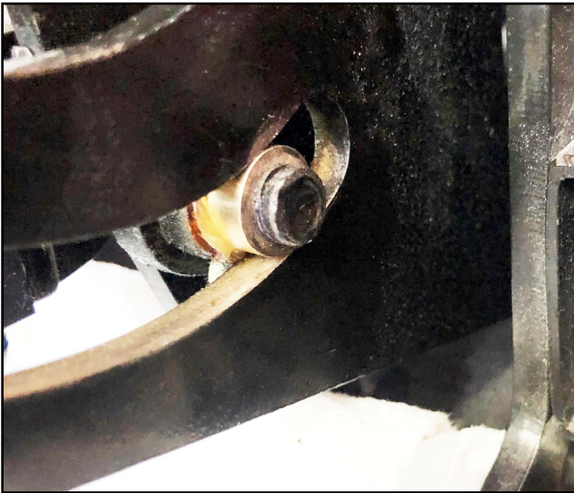
Replacement bronze bushing should move freely along entire groove.
