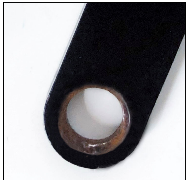
Close up of fulcrum arm with factory bushing removed
